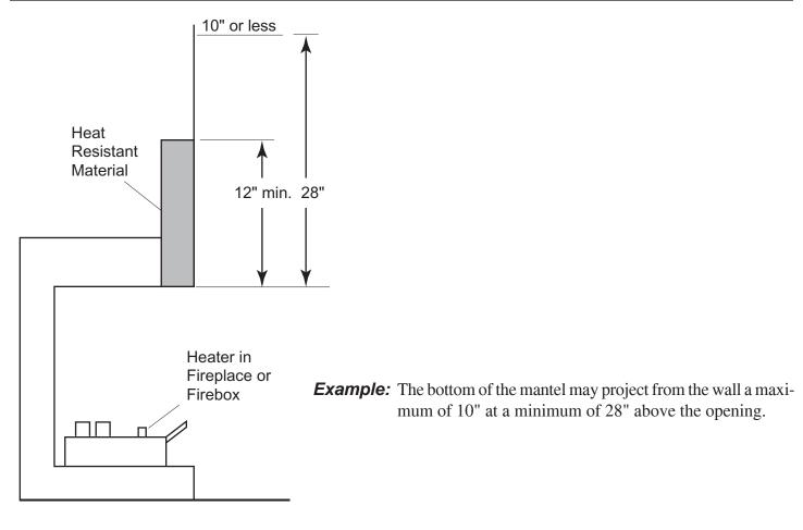
Figure 9 - Minimum Mantel Clearance with No Hood — NB24
